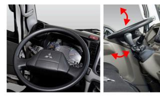
The tilt and telescopic adjustable steering wheel and in-dash gear shift lever for optimum driving position
