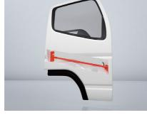
Side impact beams built into the doors strengthening door frame and rigidity to protect the driver and passengers.
