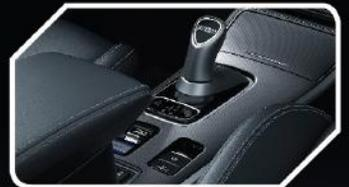
The joystick-type shift knob, 4WD selector and switches for SPORT Mode, Save/Charge Mode & ECO Mode are all housed in a nifty panel within your reach.
