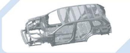
Collision safety performance is significantly enhanced by Mitsubishi Motors' RISE (Reinforced Impact Safety Evolution) body, which efficiently absorbs energy and maintains high cabin integrity in the event of a collision.
