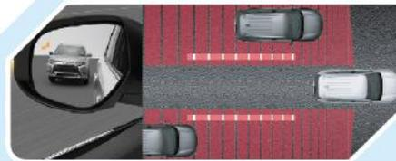
Uses radar sensors in the rear bumper to detect vehicles in your rear blind spots on both sides. An indicator appears in the door mirror when BSW is active and the turn signals are off. When a vehicle is detected while the turn signal is on, an indicator blinks in the corresponding door mirror and a buzzer sounds.
