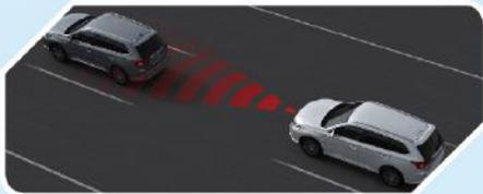
Uses radar technology to detect any cars in the lane ahead and adjusts the speed of your car accordingly while maintaining a safe distance set by you.
