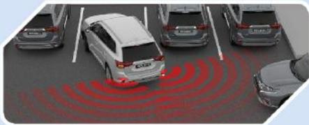
When active, an indicator appears in the combination meter display. If radar sensors in the rear bumper detect an approaching vehicle while reverse gear is engaged, a warning message appears in the multi-information display, a buzzer sounds and an indicator blinks in both door mirrors.
