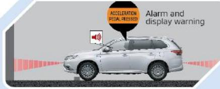
Reduces the chance and severity of hitting obstacles 4m in front or behind when a driver mistakenly presses the accelerator when stationary or at speeds up to 10 kph.
